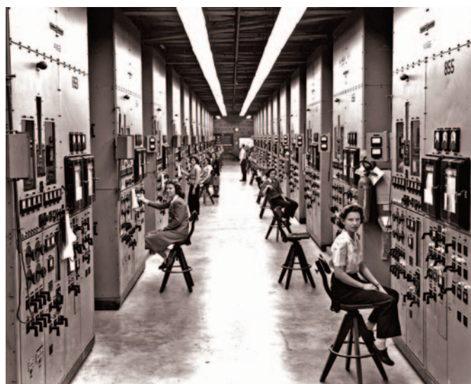
Fig 1. Mass spectrometer used for the Manhattan Project, which employed 130,000 people. Just three years after the project began, it completed its aim of developing the world’s first nuclear bomb. Various groups from across the political spectrum have called for a Manhattan Project for the Environment - a project of similar magnitude to accelerate the development of key cheap, green technologies. (Image: James E Westcott, Official US Army Photographer for the Manhattan Project / American Museum of Science and Energy.)
