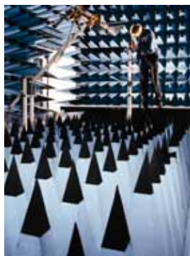
EMC testing of mobile phones. (Photo courtesy of TÜV Products Service Ltd)
